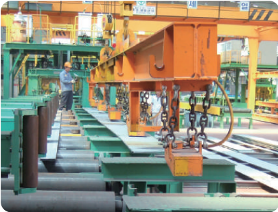
1 SUB-MATERIAL HANDLING CRANE
